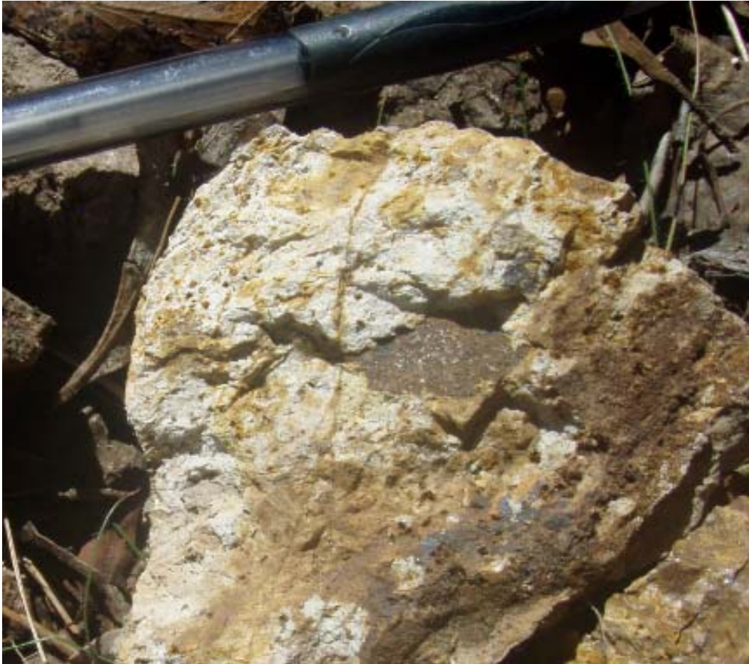
Sample S806, phyllic (quartz-sericite-pyrite) altered felsic dyke with abundant 0.5-1mm long limonite filled cubes after pyrite (location shown on Figure 1).
