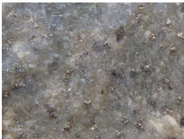
SGRDD043, 18-19m. Surface of sheeted vein alteration, studded with 0.5-2mm wide sulphides, altered felsic dyke (field of view L-R 37mm)
