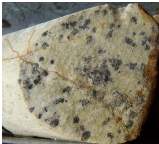
SGRDD043, 18-19m. Surface of sheeted vein alteration, studded with 0.5-2mm wide sulphides, altered felsic dyke (field of view L-R 37mm)
