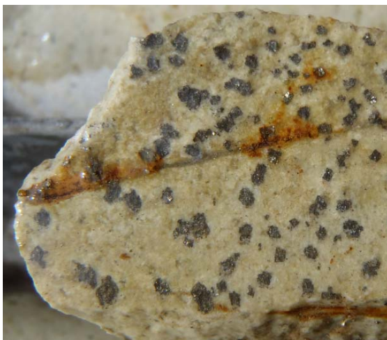
SGRDD043, 20-21m. Felsic dyke exhibiting Martins Shaft-type mineralisation. Surface of sheeted vein alteration, studded with 0.5 -2mm wide sulphides (field of view L-R 30mm)
