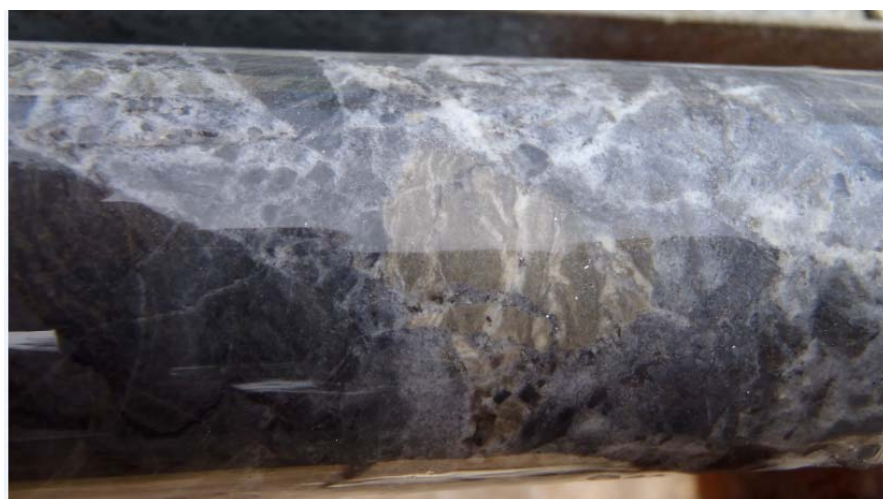
SGRDD043, 32-33m. Brecciated metasediments exhibiting quartz-sulphide-felsic dyke flooding. The light brown material (centre of core) is a finger of felsic dyke with disseminated sulphides that has forced its way through the metasediments. The simultaneous emplacement of dyke material and mineralisation is a diagnostic Intrusion-Related Gold System characteristic (field of view L-R 70mm).
