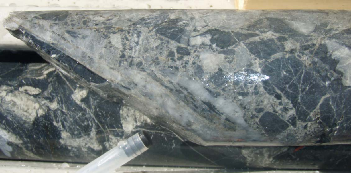
ZK001 – Brecciated metasediments flooded with sulphide-bearing felsic dyke (78-79m, NQ core 47.6mm diameter).
