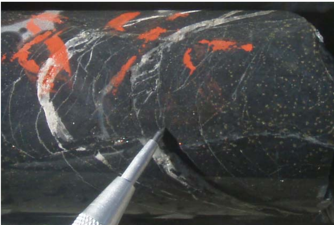
ZK001 – Sheeted veins and disseminated sulphides in metasediments (84-85m).
