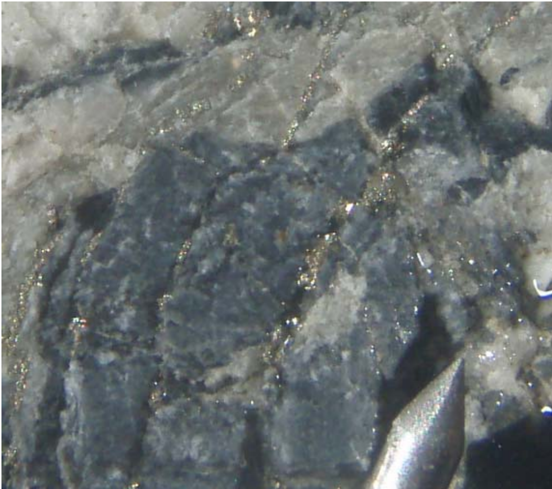
ZK001 – Stringers of light grey felsic dyke and silvery sulphides in dark grey brecciated metasediments (79-80m).
