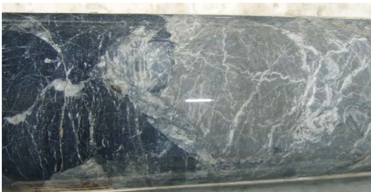
ZK001 – Core from 80-81m downhole exhibiting similar alteration and brecciation to core sample D3609 above from diamond drill hole SGRDD036. The light grey material is altered felsic dyke that has intruded the black metasediments (NQ core 47.6mm diameter).
