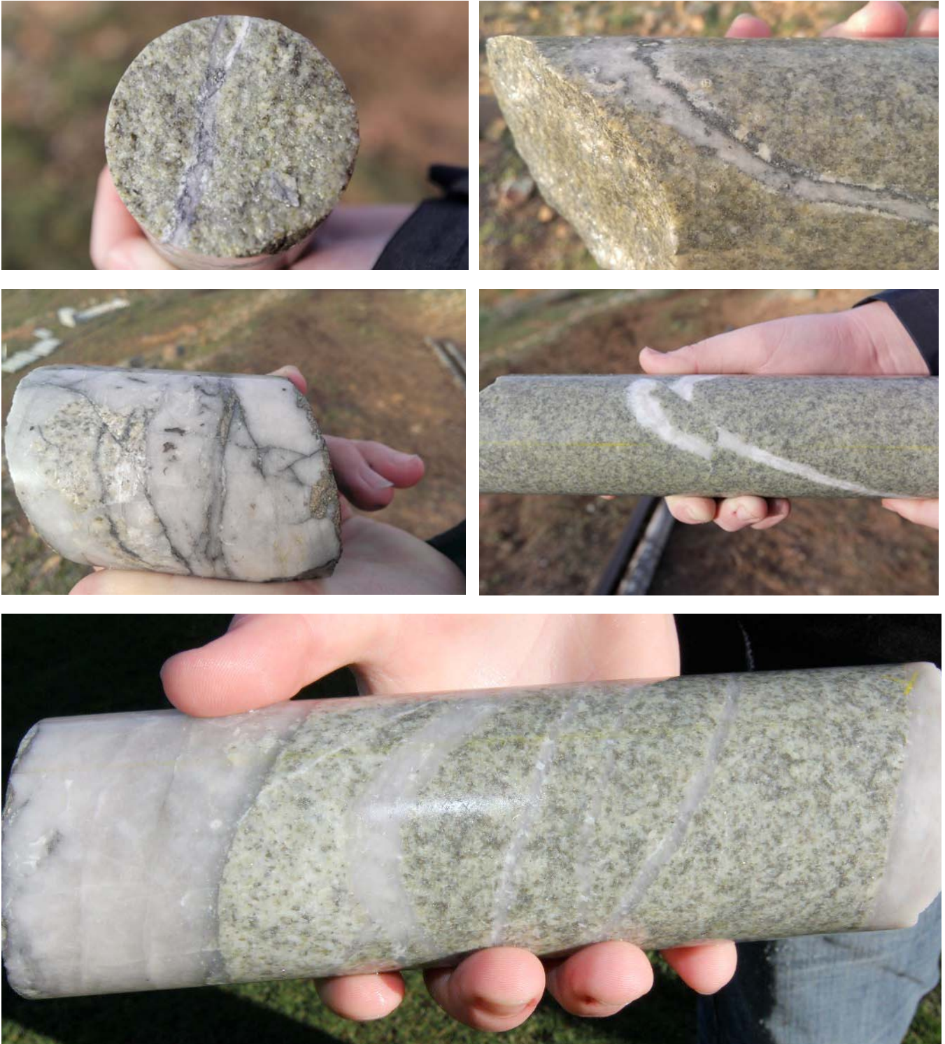
Examples of sericite-sulphide altered monzodiorite from between 300m and 770m in drill hole GHD001, with arsenopyrite-pyrite bearing quartz veins up to 10cm wide, typical of high level intrusion related gold deposits. Gold is generally associated with the arsenopyrite within the veins and disseminated throughout the rock.
