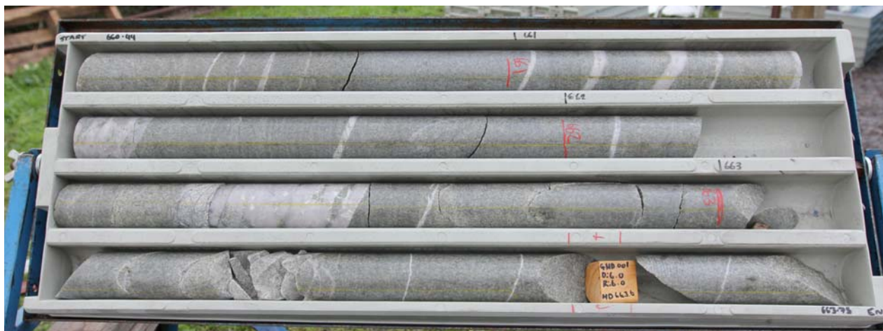
GHD001 661-664m, average 1.5g/t Au, sulphide-sericite altered monzodiorite exhibiting sheeted veins (HQ core diameter – 63.5mm)
