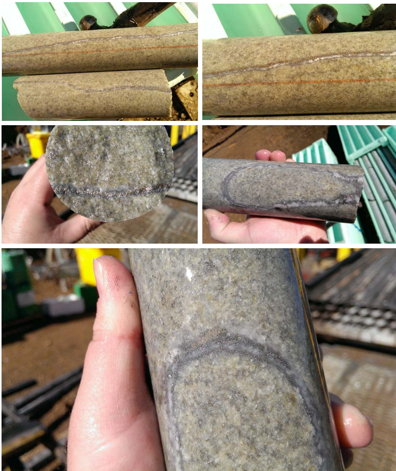
Strongly sericite altered monzodiorite, similar to higher grade core observed from hole GHD001, from approximately 630m with intense arsenopyrite-pyrite mineralisation also associated with quartz veining
