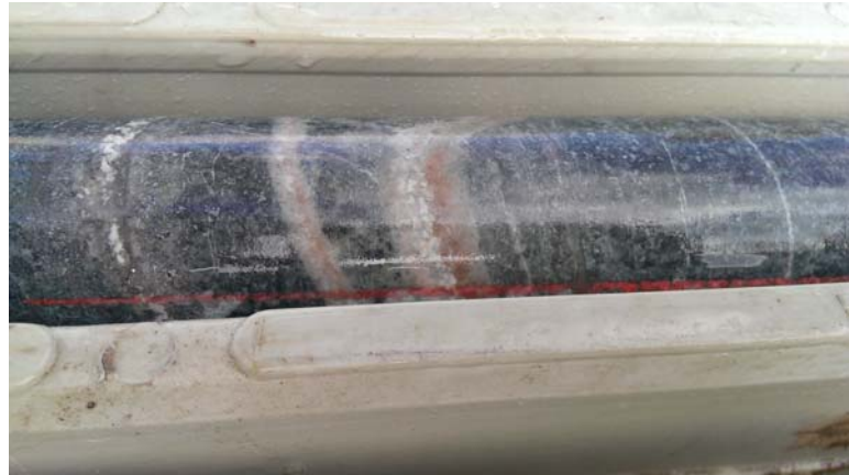
Left: Sericite altered monzodiorite near end of GHD005 and K-feldspar-quartz-carbonate vein at top right of photo
