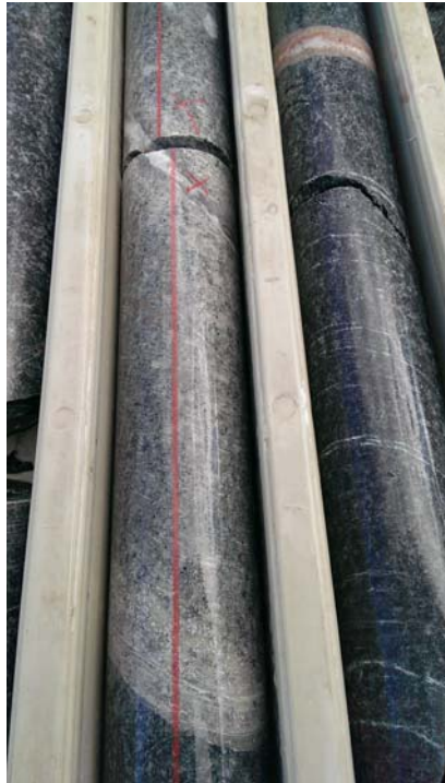
Left: Sericite altered monzodiorite near end of GHD005 and K-feldspar-quartz-carbonate vein at top right of photo
