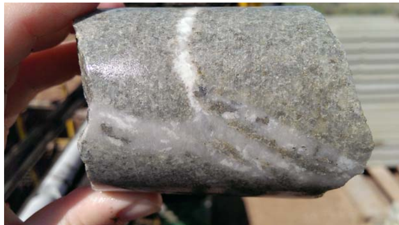
Complex multistage quartz-carbonate-sulphide tension veins in sericite-sulphide altered monzodiorite at ~557m
