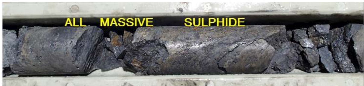
36.6 – 37.9m (approx) - all core is massive sulphide lode with very high average grade of 32.8% Zn
