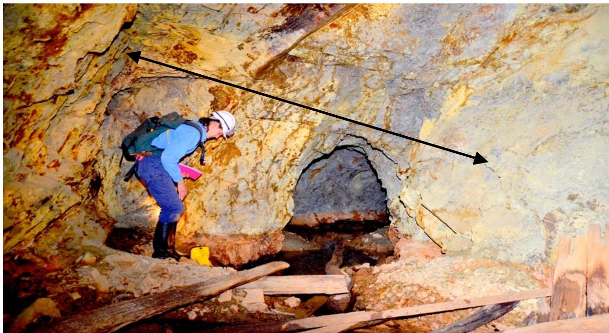
Figure 1: Southern Cross Reef Mine SW end of crosscut, Bangadang field. Composite intersection of 3m @ 7.22g/t Au; horizontal width taken across strike of mineralised structure.
