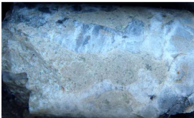
Core, SGRDD43. Black brecciated metasediments exhibiting quartz-sulphide-felsic dyke (light grey) flooding from 31.00-32.00 metres downhole, 3.93gt Au (BQ Core 36.40mm diameter).
