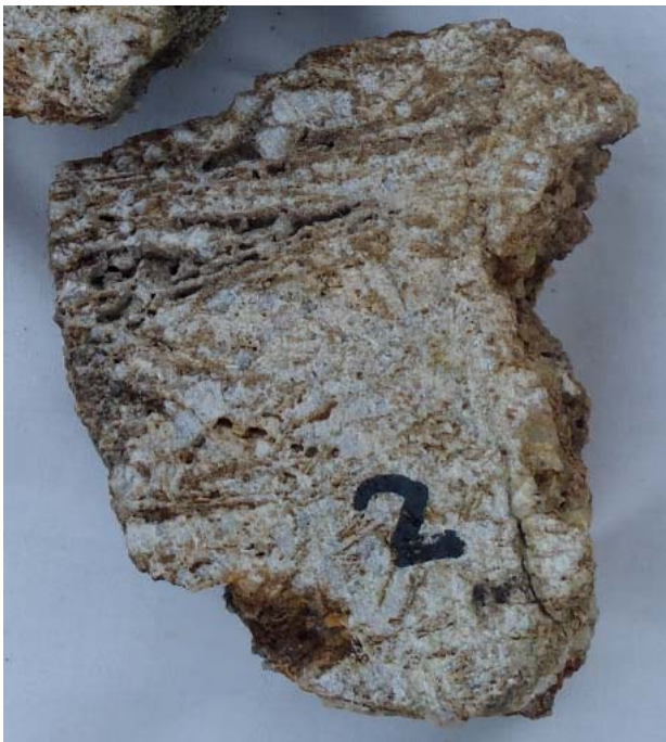
Picture 1 - Sample FFNP2, 14.85 grams/tonne Gold and 53.90 grams/tonnes Silver. Costean, Frasers Find. Portion of extensively oxidised vein comprised of prismatic and brecciated quartz associated with limonite and scorodite after sulphides. Sample: 4.2x7cm.
