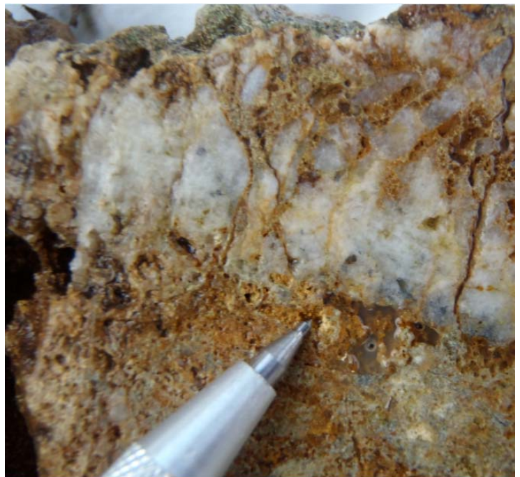
Picture 2 - Sample FFNP6, 13.50 grams/tonne Gold and 44.50 grams/tonnes Silver. Costean, Frasers Find. Portion of extensively oxidised vein comprised of prismatic and brecciated quartz associated with limonite and scorodite after sulphides. Scribe point for scale.
