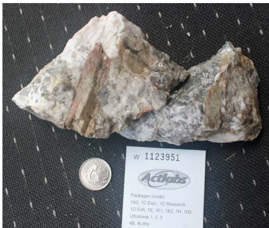
Sample 1123951: 1.09% \text{Li}_2\text{O} , from the Dempster L61 (L6100W) pegmatite. The large rectangular elongated minerals are Lithium-bearing Spodumenes.
