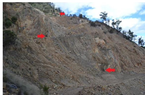
Above: Gibson mine area. The first photo with Mr Chapman was taken at the top arrow, the middle arrow is the level of the adit and the bottom arrow is where mineralisation is located below the adit
