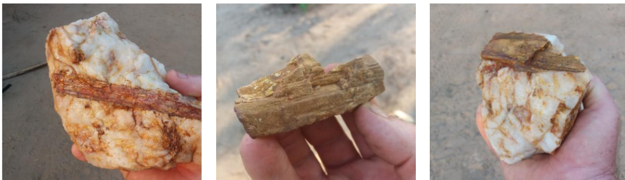
Figure 1, 2 and 3: Pegmatite hosting spodumene mineralisation identified on site at the Kitotolo Lithium Project
