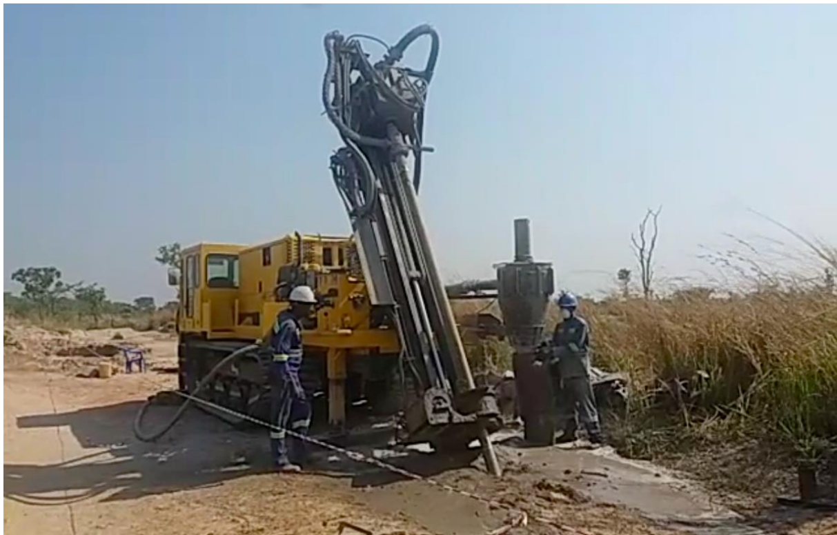
Figure 1: RC Drilling at the Kanuka Lithium Production Project in the DRC
