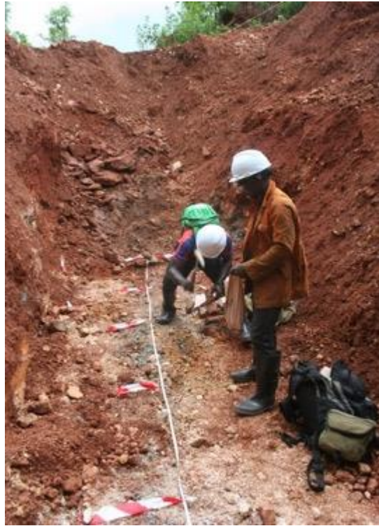
Figures 12 and 13: Commencement of Trench 003 and channel sampling exposed pegmatite at base of Trench 001.
