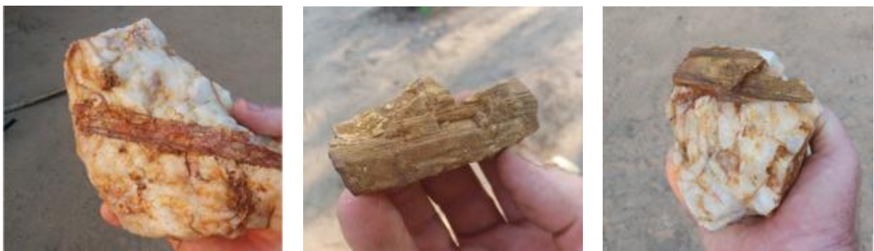
Figure 3, 4 and 5: Pegmatite hosting spodumene mineralisation at the Kitotolo Lithium Project
