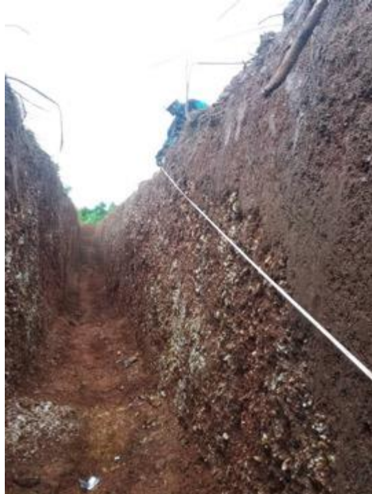
Figures 14 and 15: Trench 008 showing exposed and weathered pegmatite from surface dipping 10° to 15° west and providing upper contact structural data
