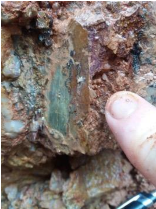
Figures 17 and 18. Partially weathered spodumene lithium mineralisation - exposed in Trench 002 and white spodumene lithium mineralisation from Test Pit 036
