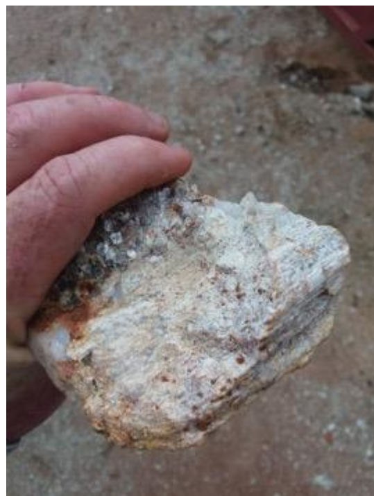
Figures 17 and 18. Partially weathered spodumene lithium mineralisation - exposed in Trench 002 and white spodumene lithium mineralisation from Test Pit 036
