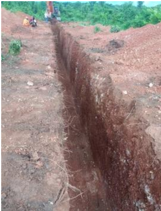
Figures 14 and 15: Trench 008 showing exposed and weathered pegmatite from surface dipping 10° to 15° west and providing upper contact structural data
