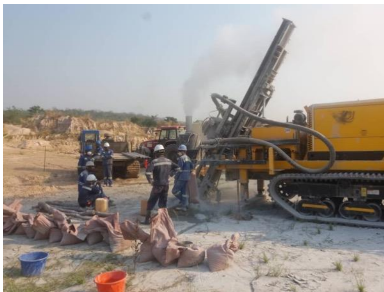
Figure 1: RC drilling at the Kanuka Lithium Production Project in the DRC
