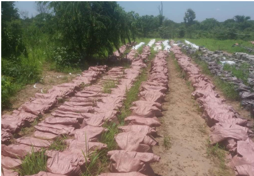
Figure 1: RC drilling samples at the Kanuka Lithium Production Project taken in the DRC in 2018
