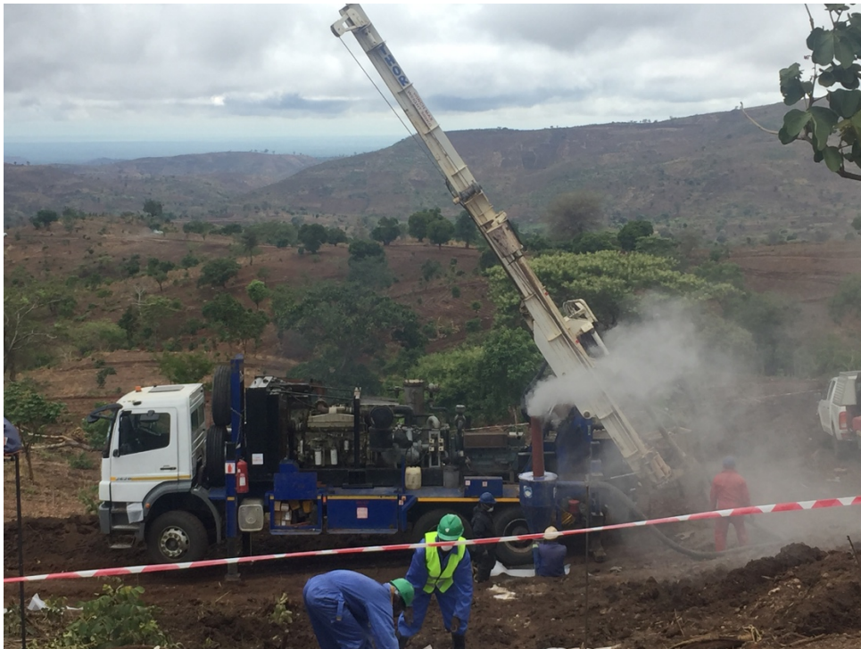
Figure 1: RC Drilling at the Small Canyon Prospect at the Tshipala Project in Malawi
