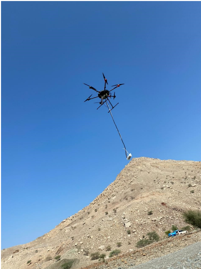
Figure 5: Drone Supported Magnetics Survey Hara Kilab
