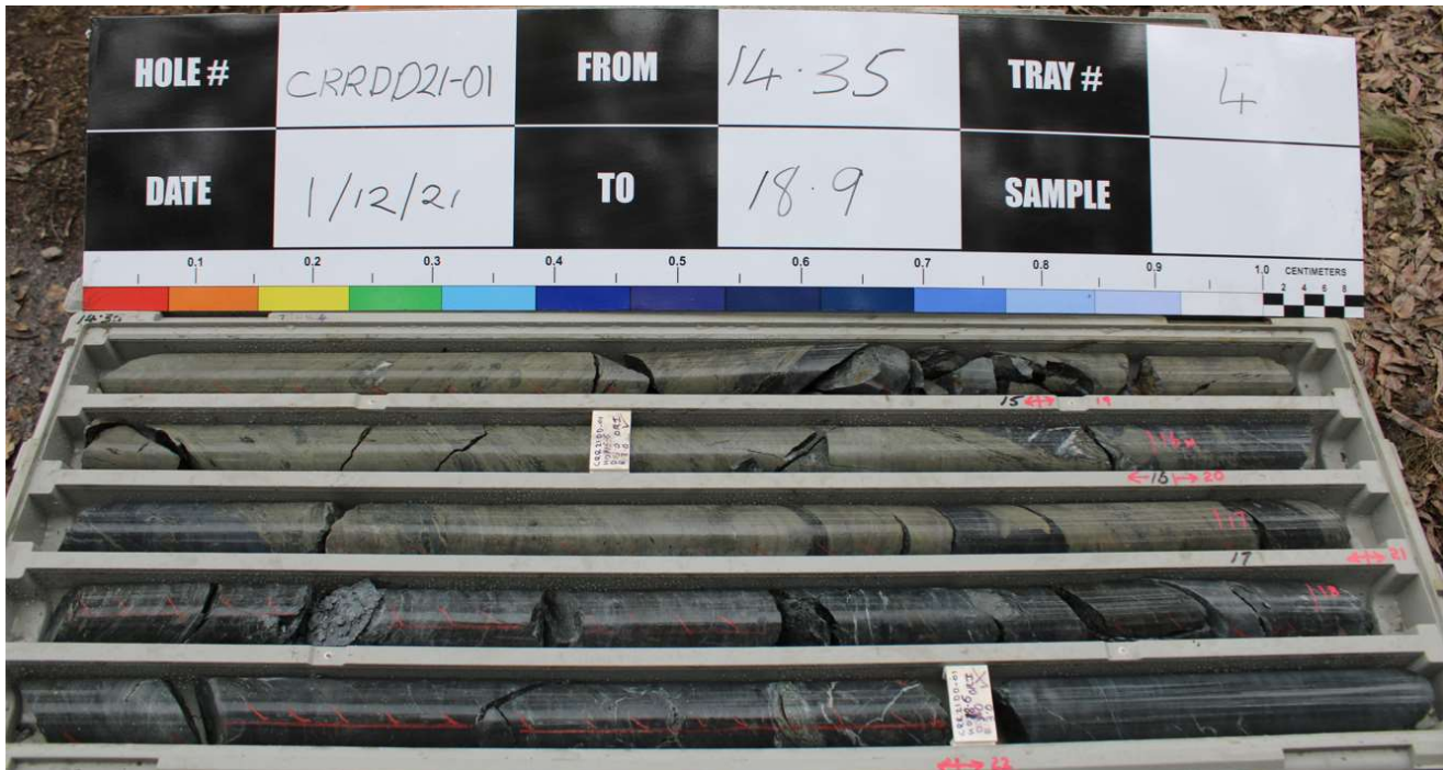
Figure 2. Core from 14.35m – 18.9m downhole, showing in the first three rows massive sulphide mineralisation that is part of a 3.8m interval (only ~ 14% black carbonaceous shales) extending from 13.3m-17.1m. (Diamond drill hole CRRDD21_01, Scale: NQ core 50mm diameter variety)
