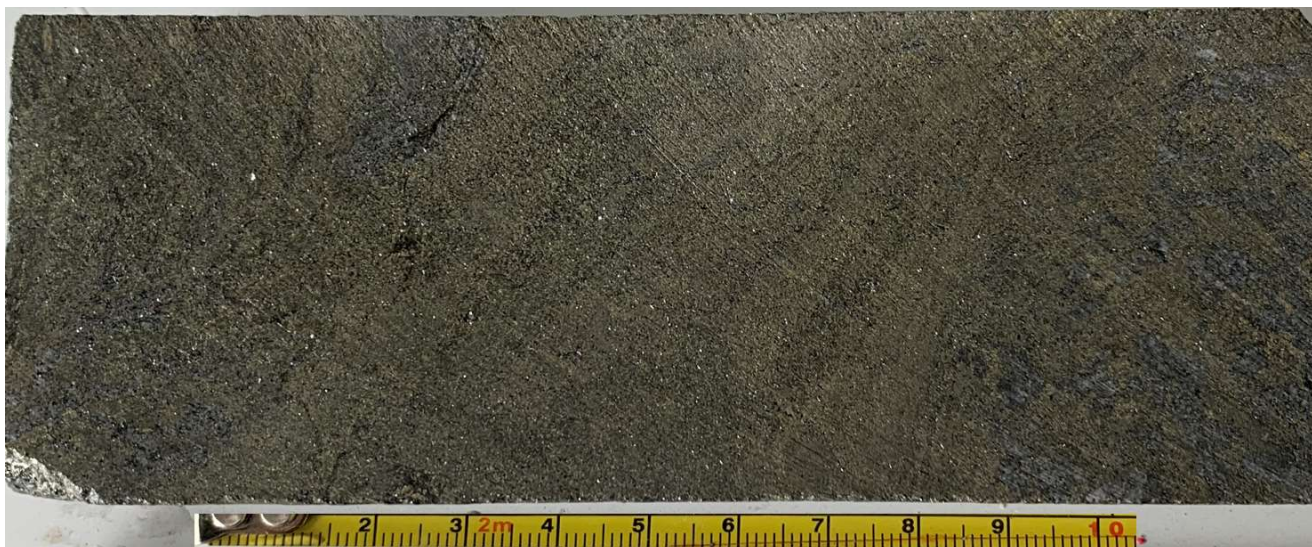
Figure 2: Detail of core from 102.8m-102.94m showing polymetallic mixed sulphides comprising sphalerite (Zinc), galena (Lead-Silver), chalcopyrites (Copper), (scale: centimetres)
