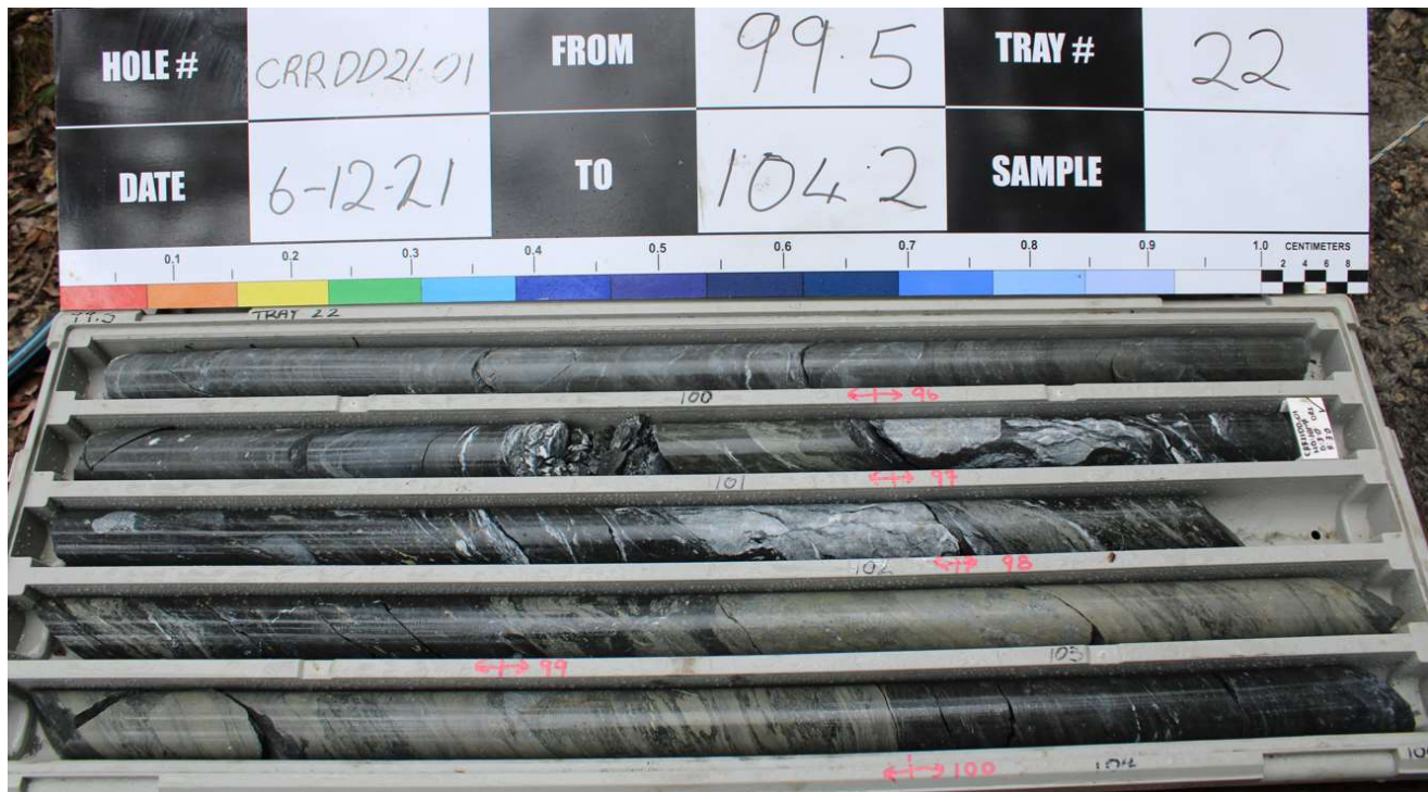
Figure 2: Detail of core from 102.8m-102.94m showing polymetallic mixed sulphides comprising sphalerite (Zinc), galena (Lead-Silver), chalcopyrites (Copper), (scale: centimetres)
