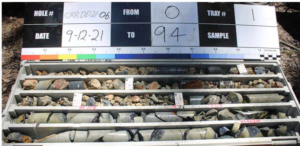
Figure 1: Diamond drill core showing (bottom three rows) part of a shallow polymetallic massive sulphide interval that extends from 7.7m-9.6m downhole - it is part of a broader highly mineralised zone of 5.3m (7.7m-13m downhole). The interval will comprise sphalerite (Zinc), galena (Lead-Silver) and chalcopyrites (Copper), (Diamond drill hole CRR21DD_06, Scale: NQ core 50mm diameter variety)
