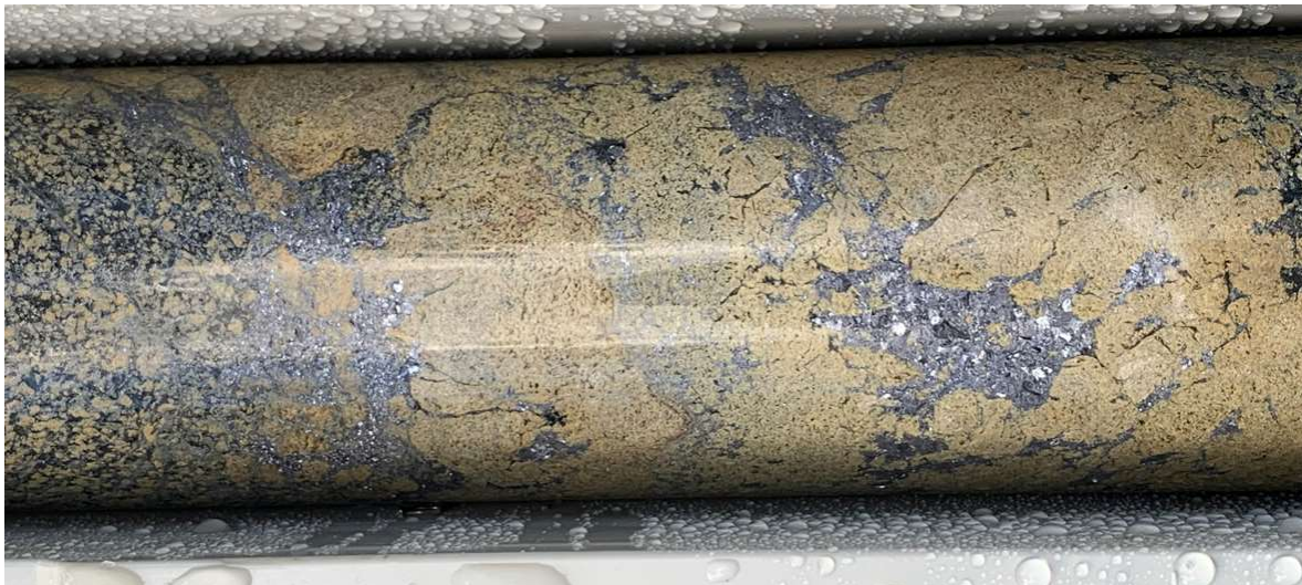
Figure 5: Detail of part of a shallow highly mineralised zone that extends from 7.7m-13m downhole. Note the yellow-brown and silvery intervals of polymetallic high grade massive sulphides that will comprise sphalerite (Zinc), galena (Lead-Silver) and chalcopyrites (Copper), (Diamond drill hole CRR21DD_06, Scale: NQ core 50mm diameter variety)
