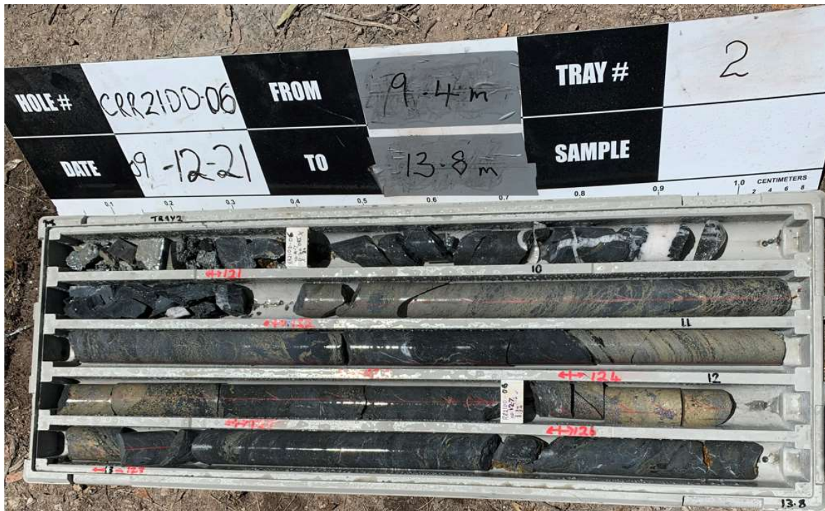
Figure 5: Detail of part of a shallow highly mineralised zone that extends from 7.7m-13m downhole. Note the yellow-brown and silvery intervals of polymetallic high grade massive sulphides that will comprise sphalerite (Zinc), galena (Lead-Silver) and chalcopyrites (Copper), (Diamond drill hole CRR21DD_06, Scale: NQ core 50mm diameter variety)
