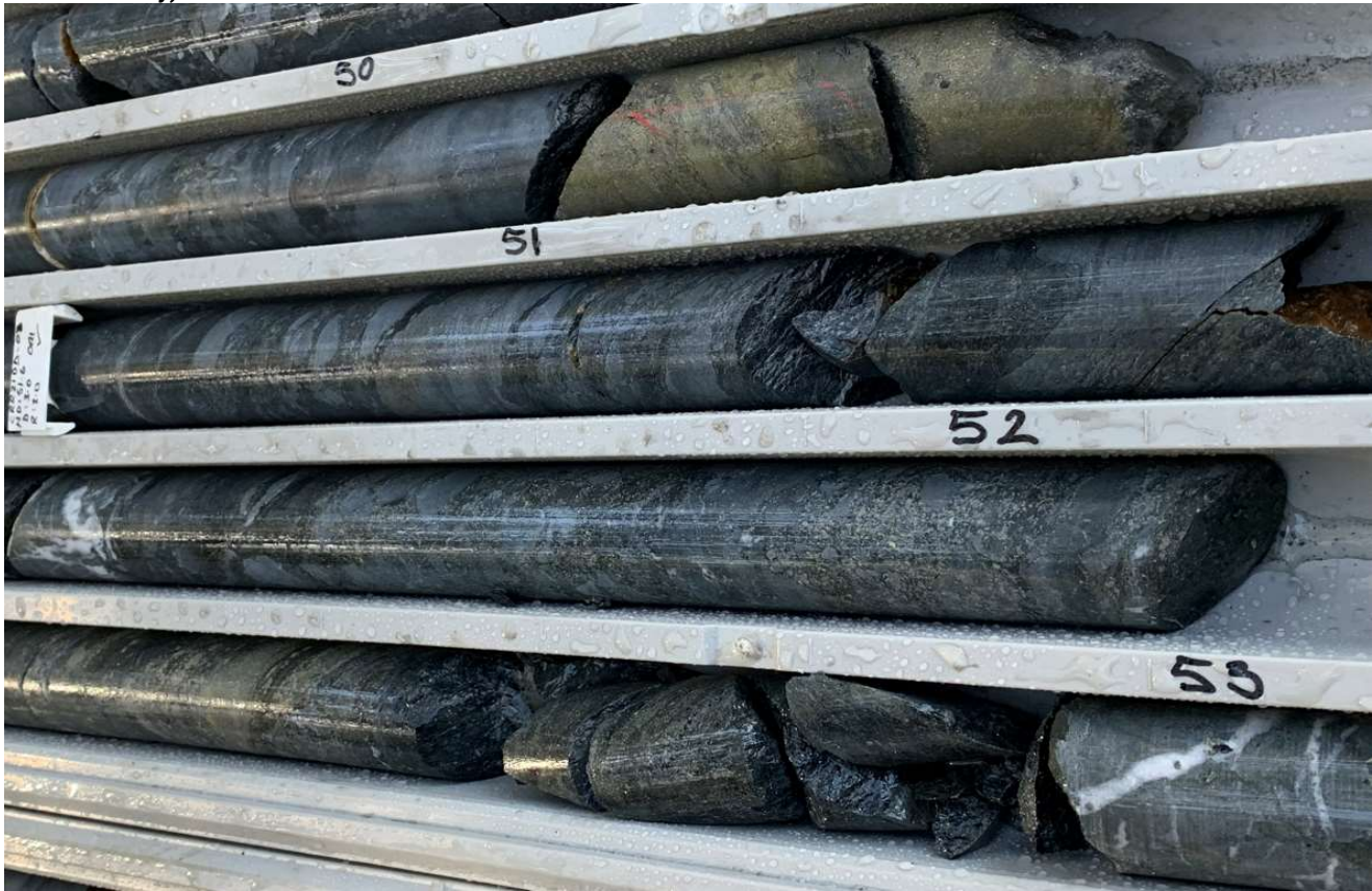
Figure 2: Detail of massive sulphide interval in photo above showing chalcopyrite (copper-iron sulphide, golden coloured, mostly LHS), sphalerite (zinc sulphide [low iron variety], yellow brown coloured, mostly RHS), galena (lead sulphide, silver coloured) and pyrite (bronze coloured) (Diamond drill hole CRR21DD_08, Scale: NQ core 50mm diameter variety)
