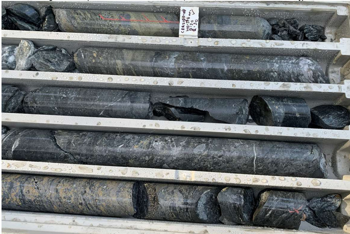
Figure 5: Disseminated sulphide mineralisation present as yellowy-brown discontinuous foliations and blebs black carbonaceous pelites (interval ~ 27.8m-30.6m downhole) (Diamond drill hole CRR21DD_08, Scale: NQ core 50mm diameter variety)
