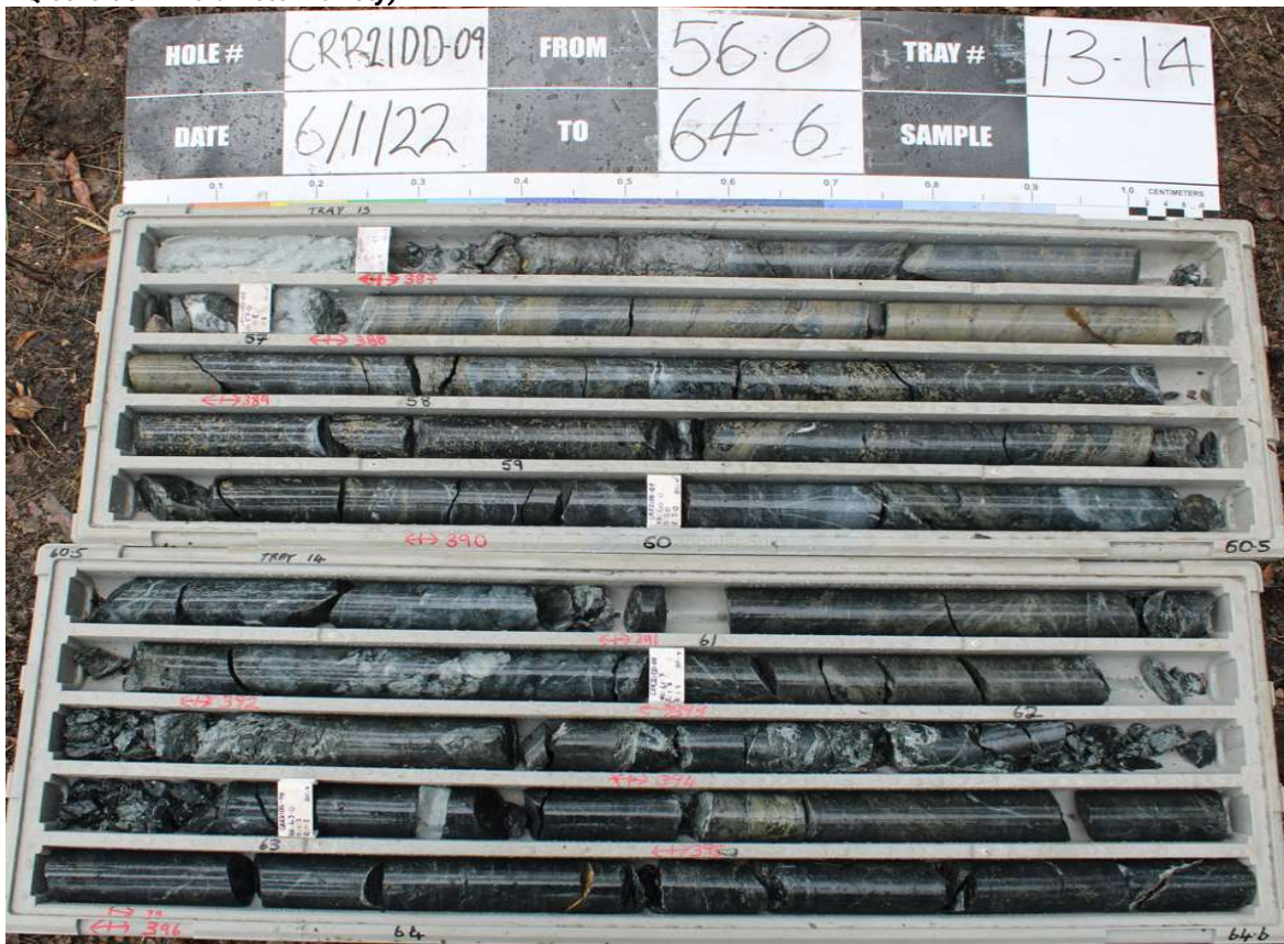
Figure 1: Core showing mineralised interval from 56.2m – 61.5m (downhole), (Diamond drill hole CRRDD21_09, Scale: NQ core 50mm diameter variety)
