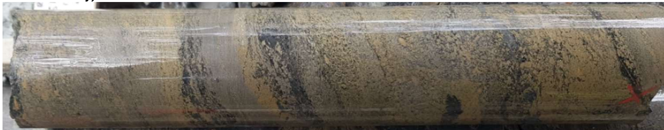
Figure 3: Section of core from 57.05-57.8m with an estimated 55-60% massive base metal sulphide (yellow-brown sphalerite and lesser galena) (Diamond drill hole CRRDD21_09, Scale: NQ core 50mm diameter variety)
