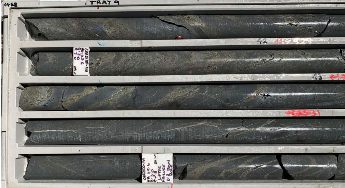
Figure 5: Detail of core with intervals of sheeted veins and stockwork mineralisation with pyrite and lesser chalcopyrite, from first five rows of tray 9 in Figure 3 above (Diamond drill hole CRR21DD_011A, Scale: NQ core 50mm diameter variety)
