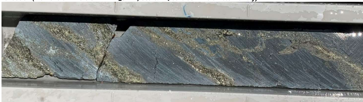
Figure 6: Half core from third row of above Figure 5, Sample 530 from 43.04-43.86m @ 1.61% Cu, 0.51% Zn, 0.03% Pb, 149g/t Ag, 0.02g/t Au. Note RHS sheeted, parallel vein, chalcopyrite at times is present towards the central portion of the sheeted veins with more pyrite towards the margin, this could be indicative of a later stage vein parting event by more copper-rich fluids. Note: Core is sawn in half:- half core sent for assay and half core retained for study and future JORC validation (Diamond drill hole CRR21DD_011A, Scale: NQ core 50mm diameter variety)
