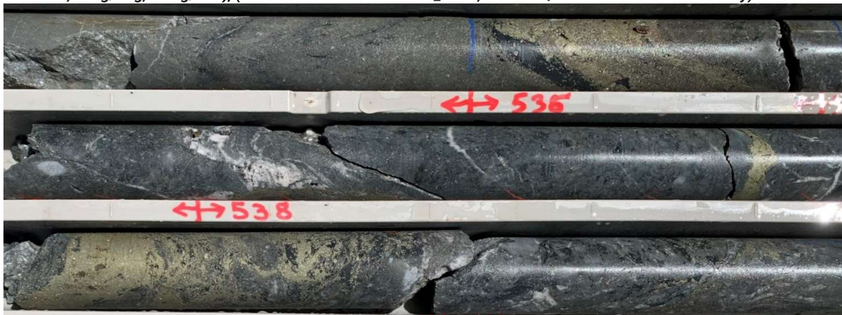
Figure 4: Detail of core with intervals of visible chalcopyrite and lesser pyrite, from first three rows of tray 10 in Figure 3 above that extend downhole from 46.2-48.7m. Top row RHS has portion of sample 536 (46.52-46.74m @ 3.30% Cu, 0.27% Zn, 0.019% Pb, 199.0g/t Ag, 0.02g/t Au;) and bottom row LHS has sample 539 (47.92-48.30m @ 6.89% Cu, 0.63% Zn, 0.01% Pb, 262g/t Ag, 0.02g/t Au), (Diamond drill hole CRR21DD_011A, Scale: NQ core 50mm diameter variety)
