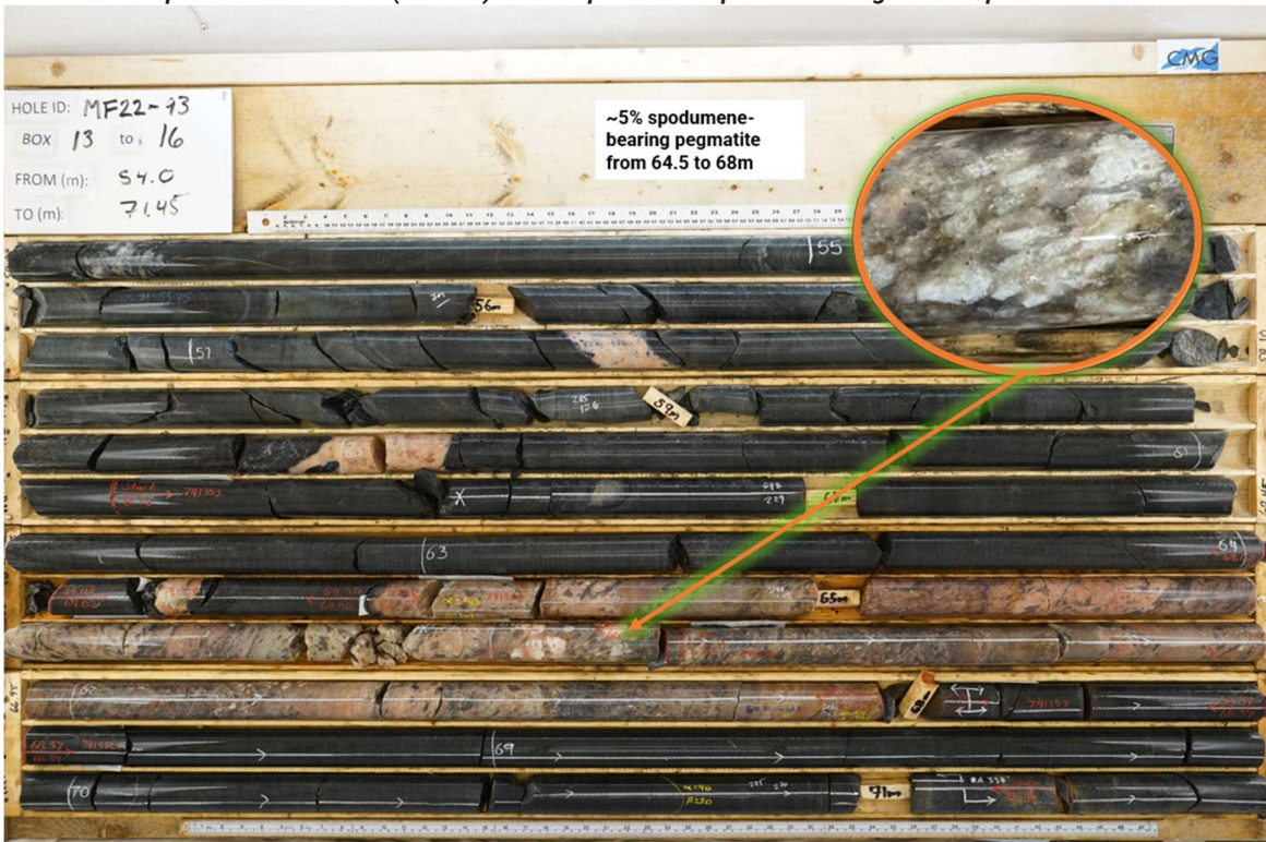
Figure 5: White pegmatite hosts approximately 5% of fine to large, white-grey, spodumene crystals intersected from 64.5 to 68m depth in Hole MF22-93 (Hole 34). Close-ups illustrate presence of significant spodumene
