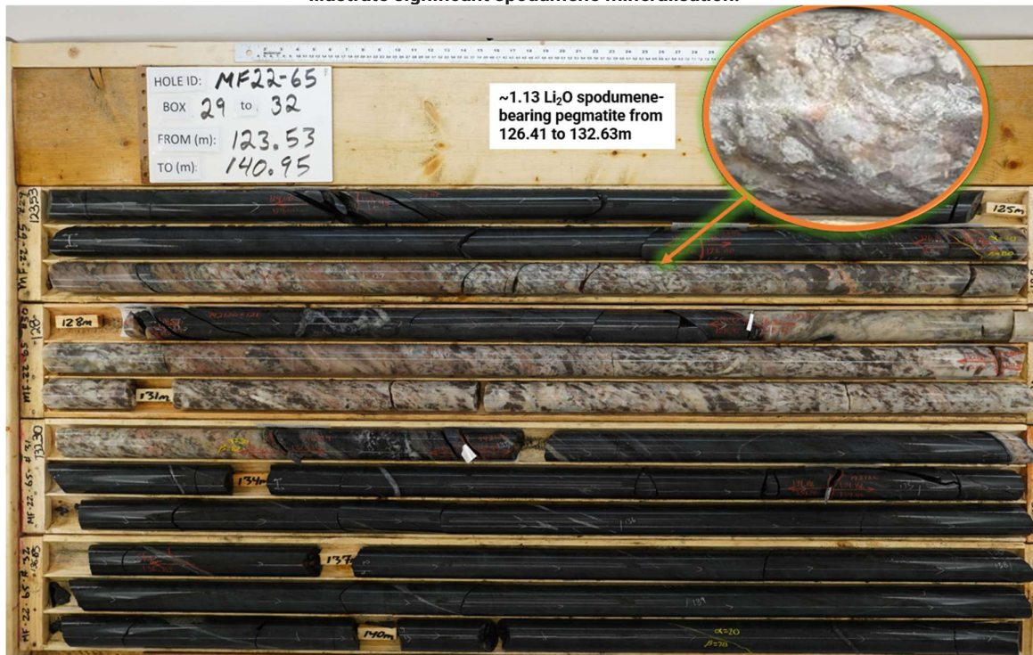
Figure 4: White pegmatite hosts spodumene laths intersected from 126.41 to 132.63m depth in Hole MF22-65. Close-ups illustrate significant spodumene mineralisation.
