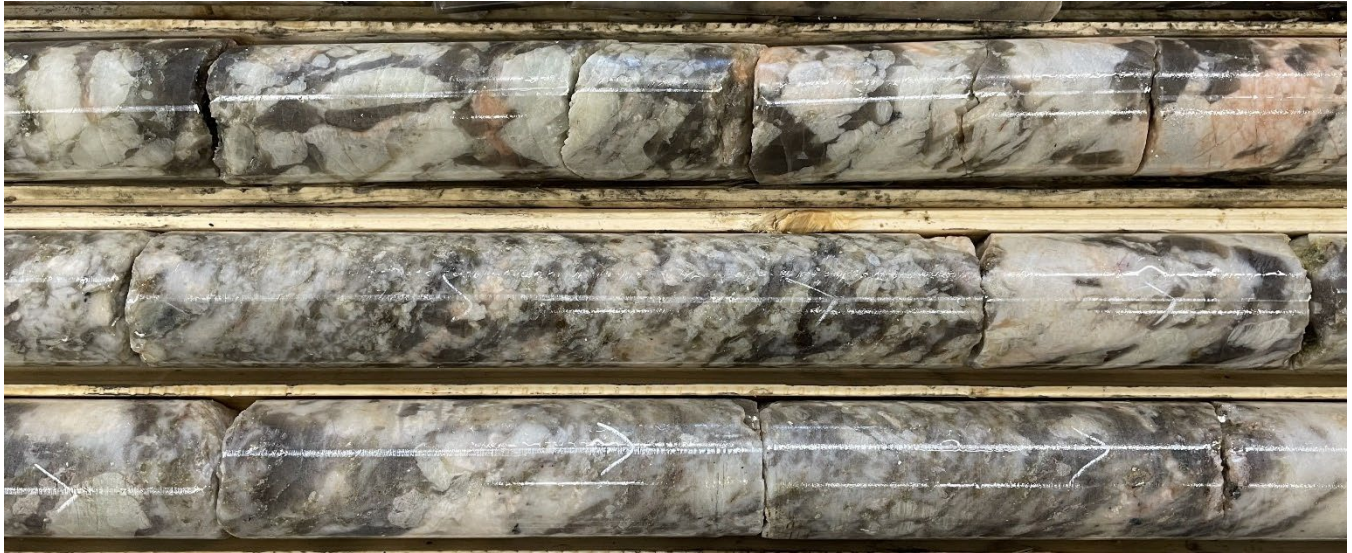
Figure 2: Close up of large white spodumene laths within the zone of MF22-123 from 50.9 to 57.15m downhole
