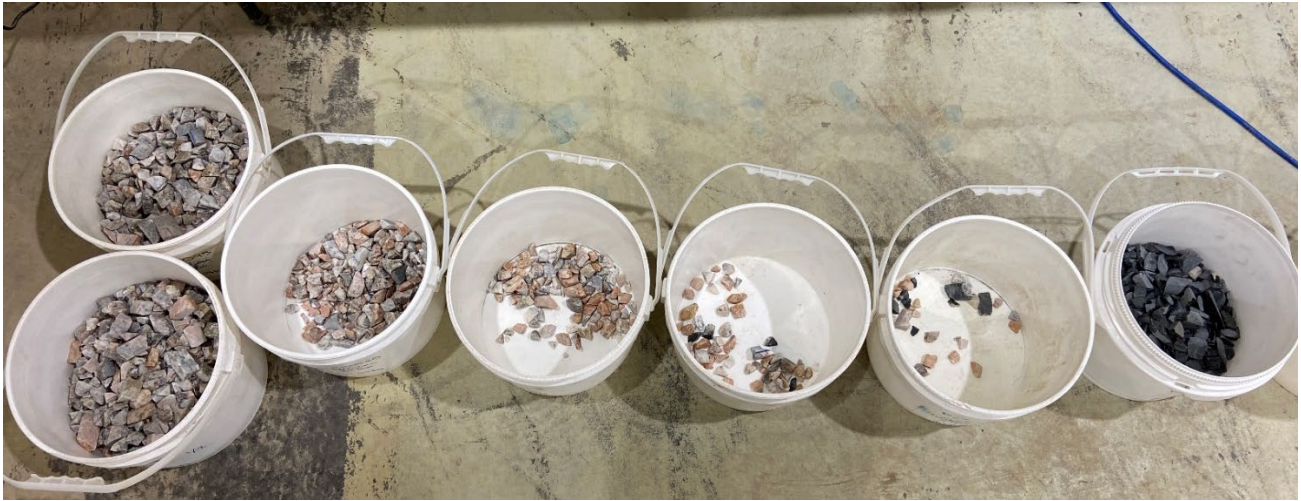
Figure 1 - Dynamic XRT ore sorting results showing separation of pegmatites (left) from waste rock (right)
