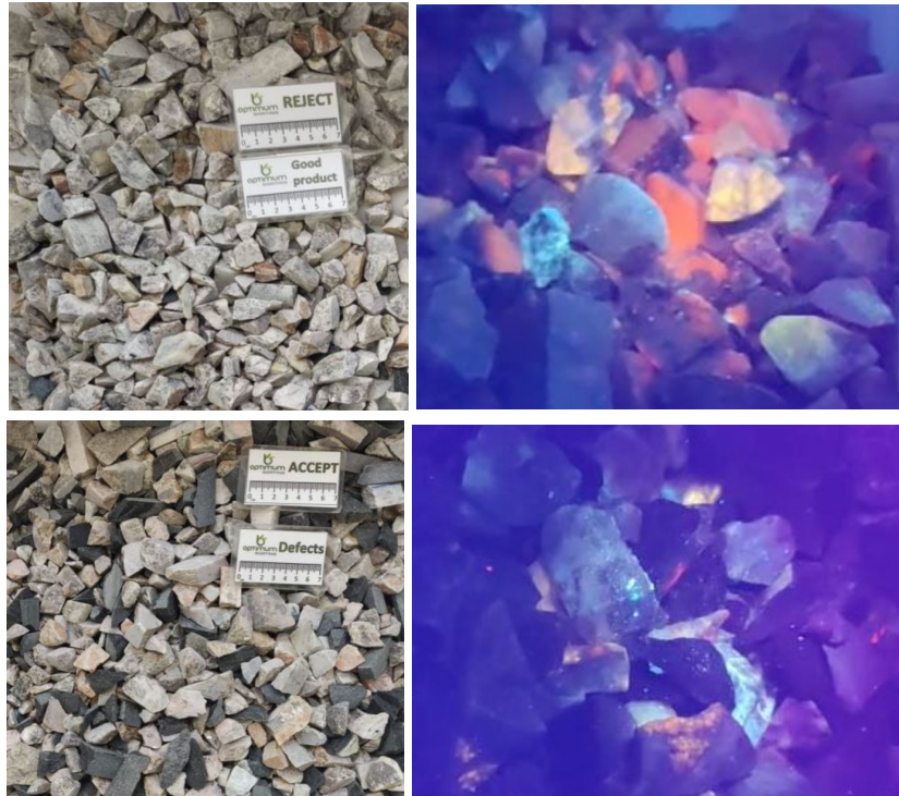
Figure 2 - Dynamic UV ore sorting trial results showing spodumene ore concentrate with its characteristic UV response (top) and waste minerals with no response (bottom)
