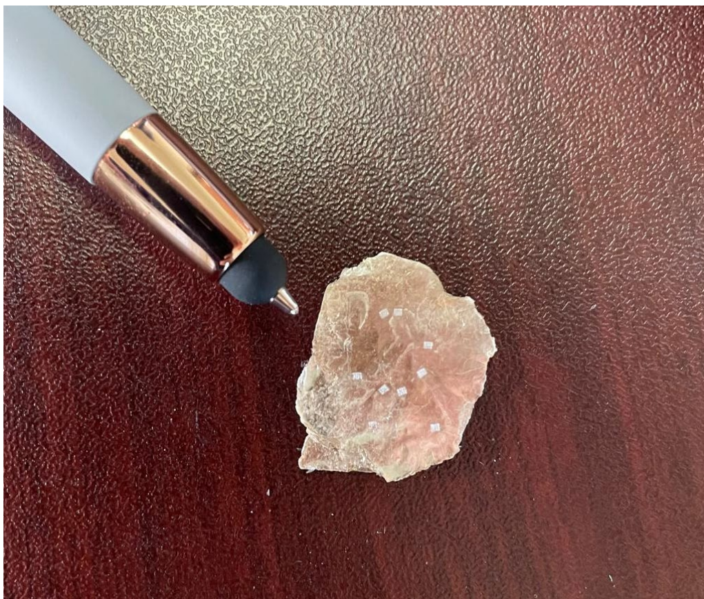
Figure 4 – Muscovite sample tested for fractionation trend using LIBS analysis
