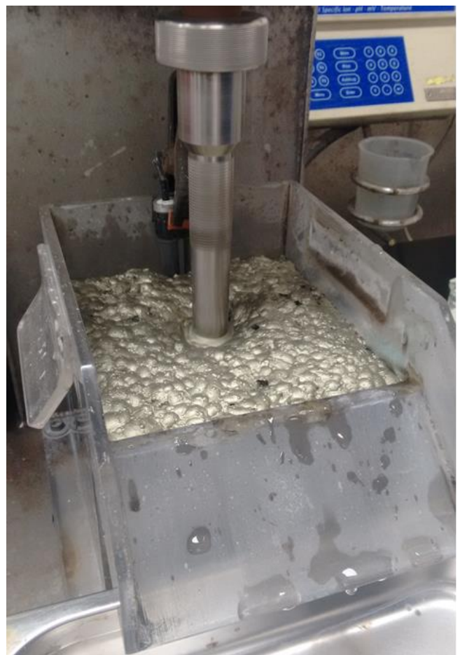
Figure 1: Flotation Testing of ore from Rover 1
