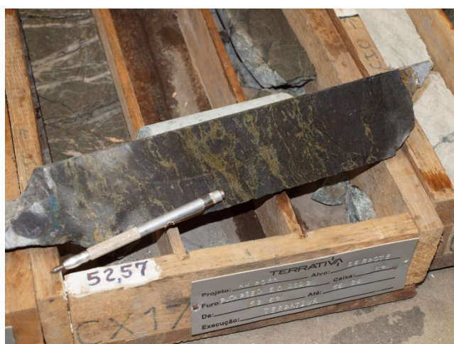
Figure 5: Left - Terrativa DDH PJCA-PSED-SD0002 (50.0-53.9 metres – 1.08% Cu); Right - Terrativa DDH PJCA-PSED-SD0004 (109.0-110.0 metres – 2.13% Cu)
