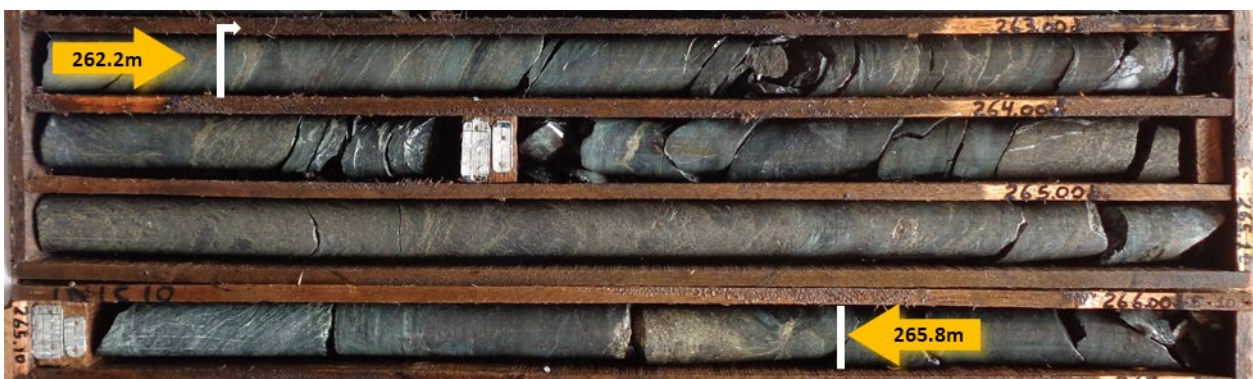
Figure 12 – Core photos from drill hole JAG-DD-20-45 (Onça Rosa); 262.2 to 265.8m: Semi-massive to massive sulphides (metallic bronze/yellow colour) with intense magnetite (black colour) mineralisation hosted in altered granite. Sulphides comprising pyrite, pentlandite, millerite and minor chalcopyrite. Assays awaited
