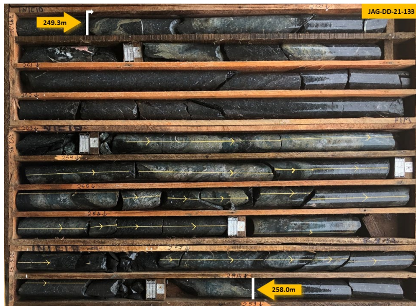
Figure 11 – Core photo from drill hole JAG-DD-21-133 (Jaguar Central); 249.3m to 288.9m down-hole. Disseminated, stringer to semi-massive sulphides (metallic bronze/yellow colour) with magnetite (black colour) mineralisation hosted in altered dacite. See Table 2 for sulphide content description.
