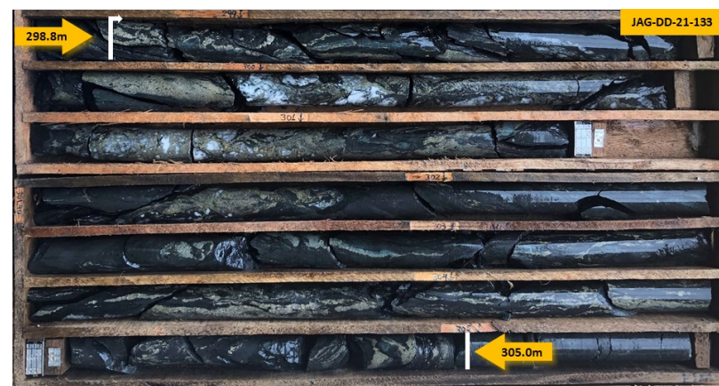
Figure 12 – Core photo from drill hole JAG-DD-21-133 (Jaguar Central); 298.8m to 305.0m down-hole. Disseminated, stringer to semi-massive sulphides (metallic bronze/yellow colour) with magnetite (black colour) mineralisation hosted in altered dacite. See Table 2 for sulphide content description.
