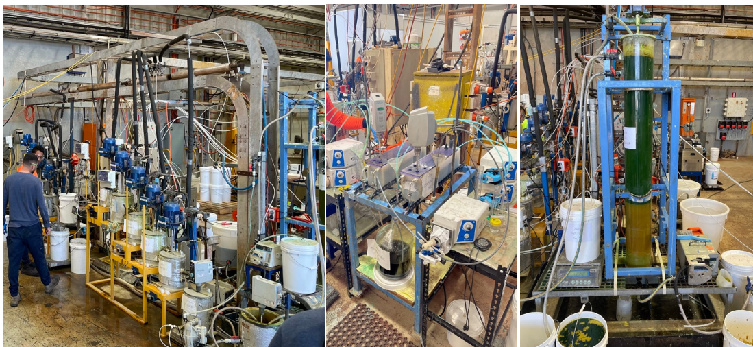
Figure 4: Primary Neutralisation, Copper Solvent Extraction and Secondary Neutralisation
