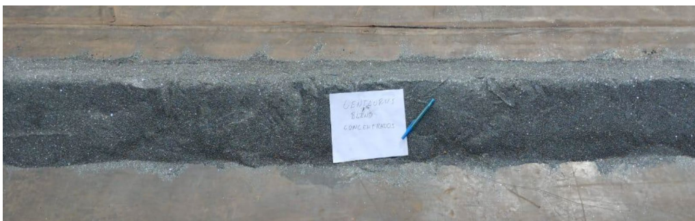
Figure 7 – Jambreiro DR-quality concentrate produced from pilot plant
