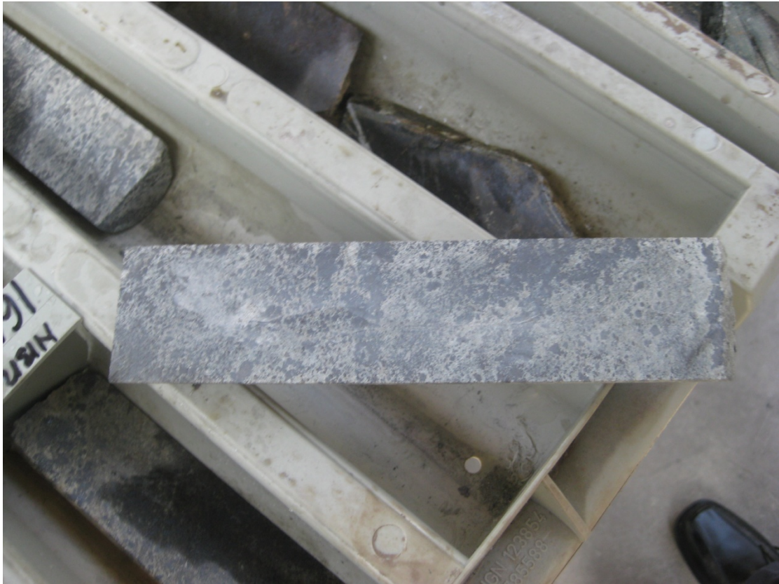
Plate 3: Sawn magnetite (coarse grained) core from Nelson Bay River Project
