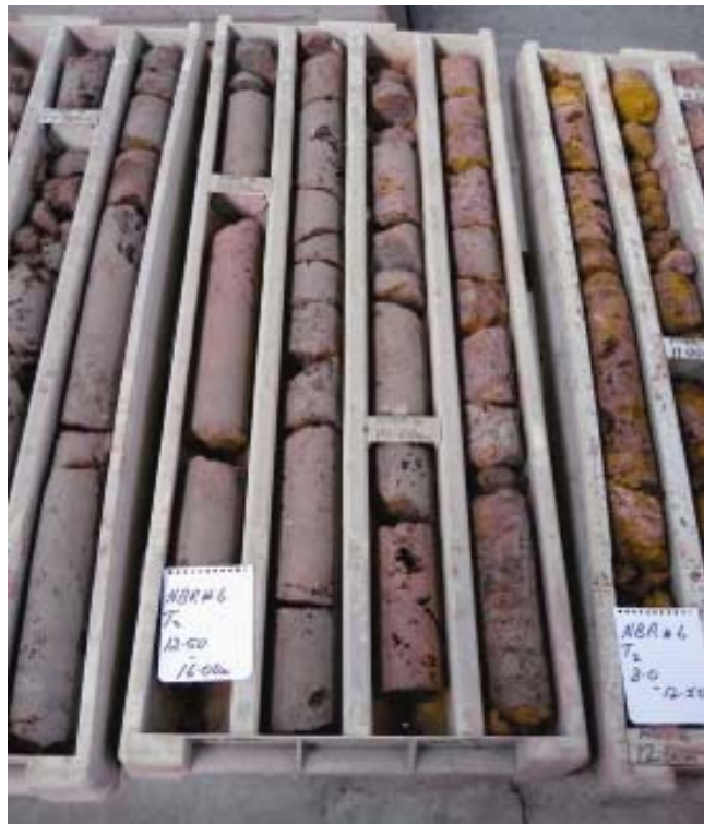
Plate 2: Goethitic hematite core from drillhole NBR-6
