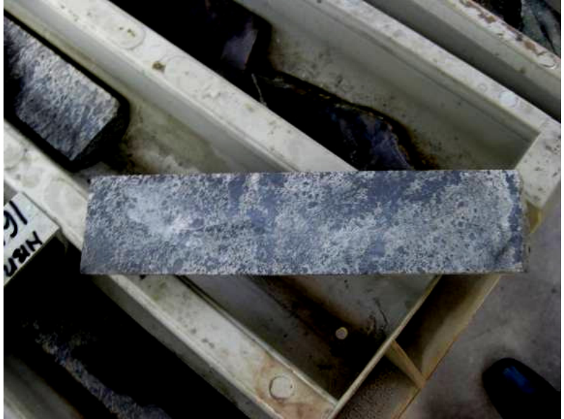
Plate 2: Core of magnetite iron ore
