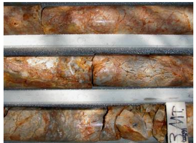
Plate 6: Stockwork veining in drillhole SCDDH5
