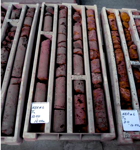
Plate 1: DSO iron ore core
