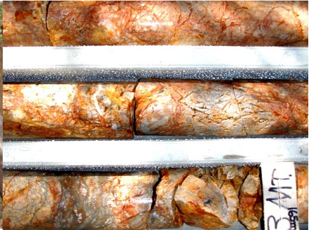
Typical stockwork veining in SCDDH5 ~165m (3m @ 1.29g/t AU)
