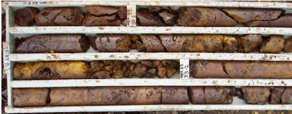
Goethitic Hematite Drill core- DSO Material
