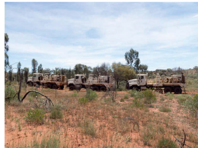
Figure: Seismic vibrator array in Southern Amadeus Basin providing energy to image sub-surface horizons
