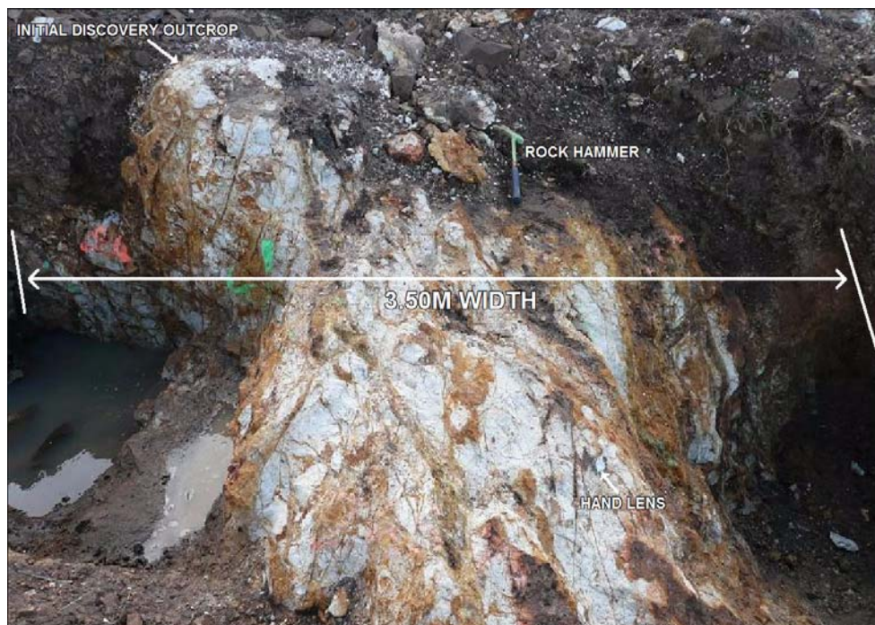
Figure 3: Altered and gossanous zone exposed in Trench 8. Assayed interval returned 3.50 metres at 3.1g/t Au, 153g/t Ag and 2.9% Pb
