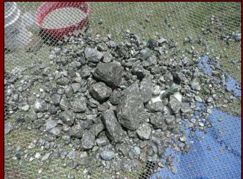
95 % massive sulphide vein MSRC11, 37-38m
