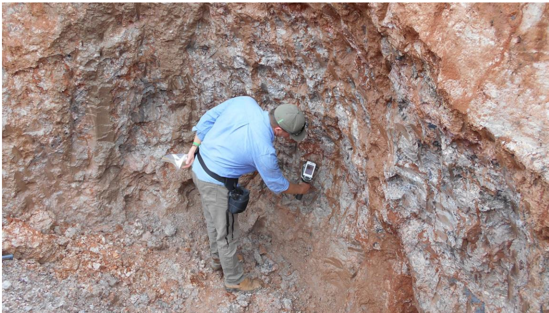
Handheld XRF analysis at Kasombo 6
