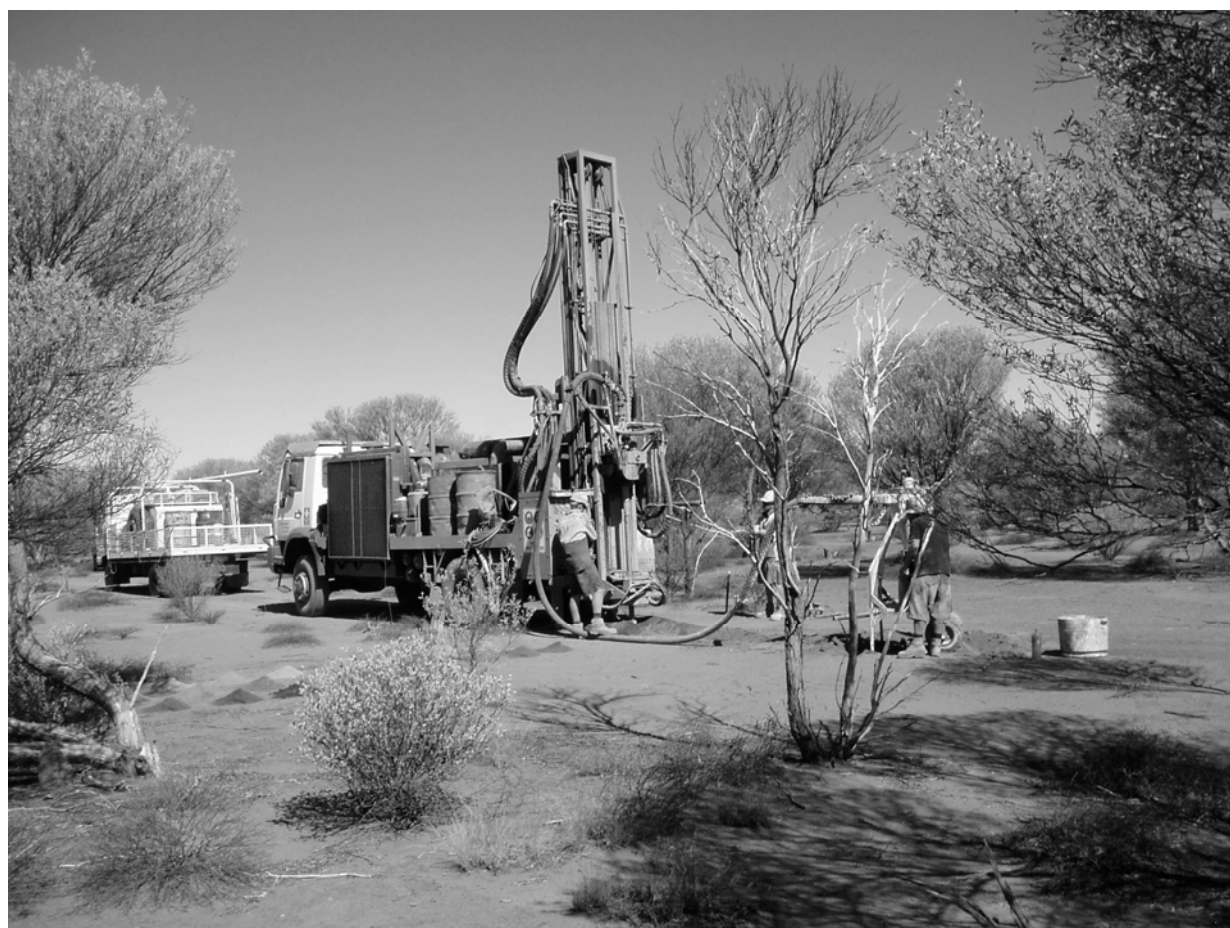
Aircore drilling at the Agnew project
