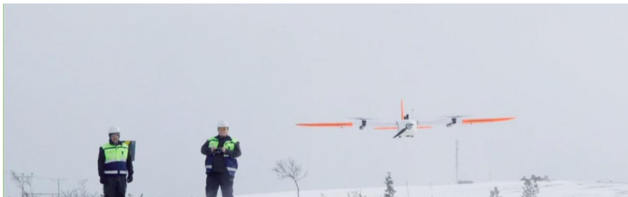
Figure 2. Drone equipment being utilized for the high-resolution magnetic survey.
