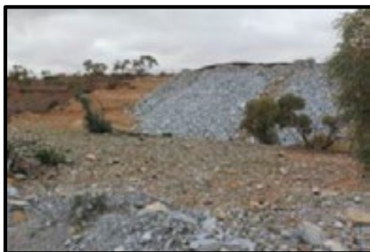
Plate 12: Waste dump in MPL 18 showing top soil removal
