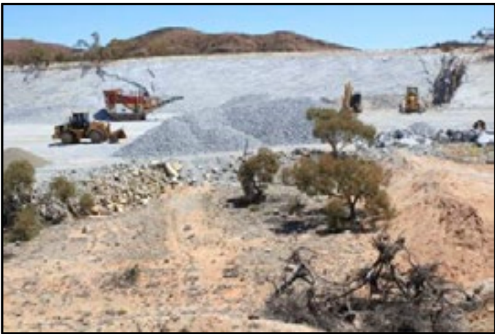
Plate 14: In pit crushing plant and crushed ore stockpiles
