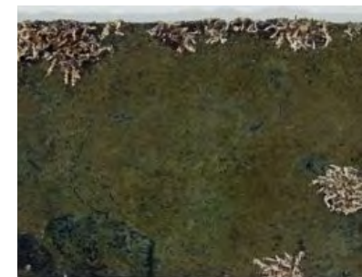
Ablative marine coating – 200 g /L Calix "bio-active" MgO
