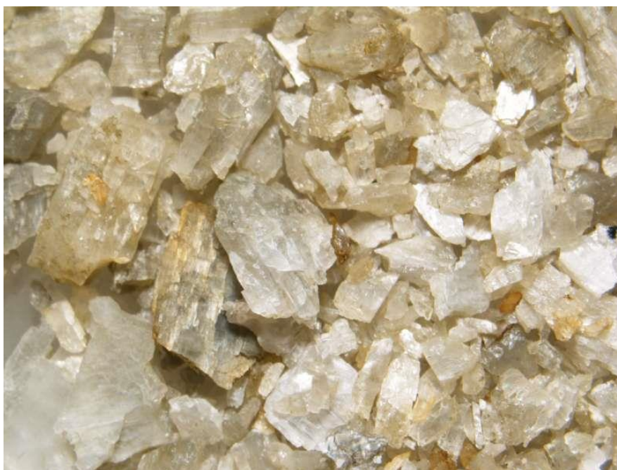
Figure 1. 8.10% Li 2 O Spodumene from HLS Testwork (SG 3.1 Sink).
